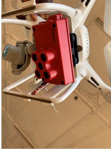
Plate 3.1: Micasense camera-equipped UAV used for aerial photography. Source: Author (2023)
